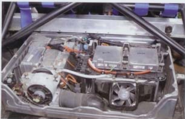
BELOW The hybrid battery and controllers in the Honda Insight
