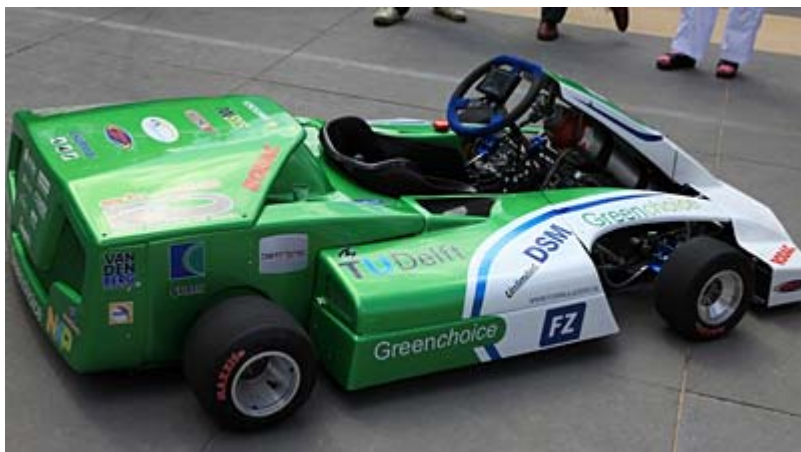
Team Delft's Formula Zero kart is made from 70 per cent bio-renewable materials Copyright ©2009 BskyB
